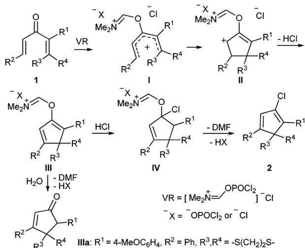
**Scheme 3** Proposed mechanism for tandem Nazarov cyclization–halovinylolation of **1** mediated by Vilsmeier reagent.
