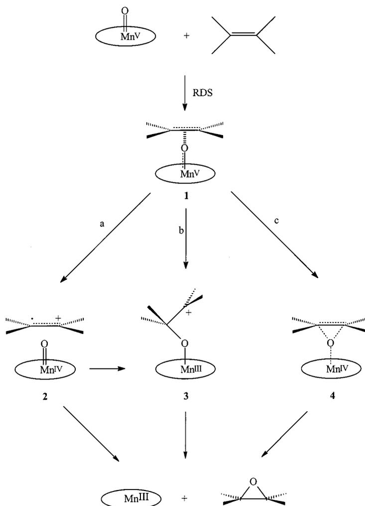
Scheme 1. Unified mechanism for the oxygen transfer from oxo-metalloporphyrins to alkenes<sup>[8]</sup>
