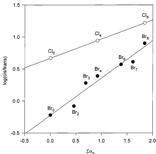
Figure 1. Correlation diagram of the logarithm of the *cis/trans* epoxides ratio vs. the sum of Hammett's  $\sigma_p$  for the epoxidation of *cis*-stilbene catalysed by a series of progressively β-halogenated MnTPPCl (filled circles) and MnTDMPPCl (open circles)
