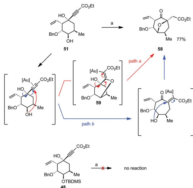
**Scheme 14** Reagents and conditions: (a)  $\text{Ph}_3\text{PAuNTf}_2$ ,  $\text{CH}_2\text{Cl}_2$ ,  $120^\circ\text{C}$ , 77%.
