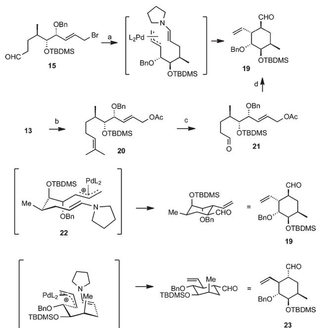
**Scheme 4** Reagents and conditions: (a) Pd(PPh<sub>3</sub>)<sub>4</sub>, pyrrolidine, THF, rt, 83%, dr = 5 : 1; (b) Ac<sub>2</sub>O, Et<sub>3</sub>N, DMAP, CH<sub>2</sub>Cl<sub>2</sub>, 91%; (c) *m*CPBA, CH<sub>2</sub>Cl<sub>2</sub>, rt; then: H<sub>2</sub>IO<sub>6</sub>, Et<sub>2</sub>O, 96%; (d) Pd(PPh<sub>3</sub>)<sub>4</sub>, pyrrolidine, DMSO, rt, 43%.
