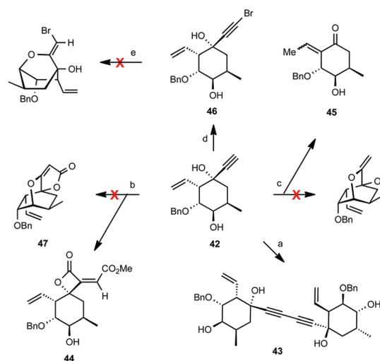
**Scheme 11** Reagents and conditions: (a)  $\text{Pd}(\text{OAc})_2$ , TMTU,  $\text{CuCl}_2$ ,  $\text{NH}_4\text{OAc}$ , propene oxide, CO, THF,  $55^\circ\text{C}$ , 50%; (b)  $\text{Pd}(\text{MeCN})_2\text{Cl}_2$ , CO, MeOH,  $\Delta$ , 77%; (c)  $\text{Ag}_2\text{CO}_3$ , benzene,  $\Delta$ , 39%; (d) NBS,  $\text{AgNO}_3$ , acetone, 85%; (e) NaOMe, MeOH,  $\Delta$ .
