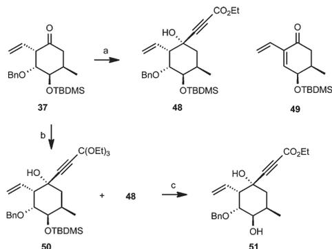
**Scheme 12** Reagents and conditions: (a) LiCCCO<sub>2</sub>Et, THF, −78 °C, 33% (89% BRSM); (b) LiCCC(OEt)<sub>3</sub>, toluene, −78 °C to rt, 88%; (c) HF, MeCN, 60 °C, 91%.
