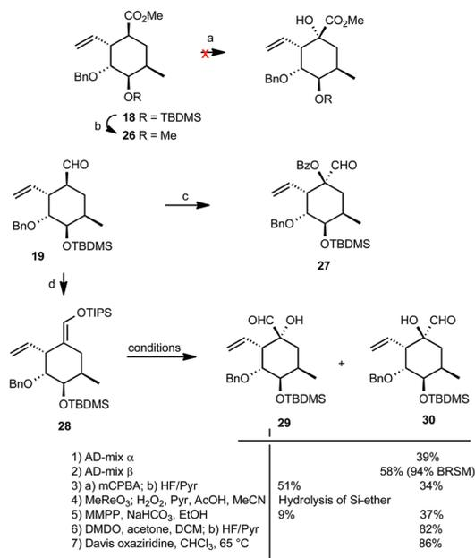
**Scheme 6** Reagents and conditions: (a)  $\text{KHMDs}$ ,  $\text{O}_2$ , THF,  $-78^\circ\text{C}$ ; then  $\text{P}(\text{OMe})_3$ ; (b) 1. HF, MeCN,  $\Delta$ , 90%; 2. NaH, MeI, THF, 64%; (c) *N*-methyl-*O*-benzoylhydroxylamine hydrochloride, DMSO,  $50^\circ\text{C}$ , 33%; (d) TIPSOTf,  $\text{Et}_3\text{N}$ ,  $\text{CH}_2\text{Cl}_2$ ,  $50^\circ\text{C}$ , 99%. TIPSOTf = triisopropylsilyl triflate; MMPP = magnesium monoporphthalate.
