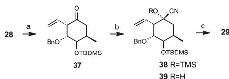
**Scheme 9** Reagents and conditions: (a)  $m\text{CPBA}$ ,  $\text{CH}_2\text{Cl}_2$ , rt; then  $\text{H}_5\text{IO}_6$ ,  $\text{Et}_2\text{O}$ , 87%; (b)  $\text{TMSCN}$ ,  $\text{ZnI}_2$ ,  $\text{CH}_2\text{Cl}_2$ , rt, 90%; on purification on  $\text{SiO}_2$  **38** was partially deprotected to give **39**; (c) DIBAL,  $\text{CH}_2\text{Cl}_2$ ,  $-78^\circ\text{C}$ ; then HCl, 50%.
