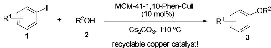
**Scheme 1.** Heterogeneous Cu-catalyzed C-O coupling between aryl iodides and alcohols.
