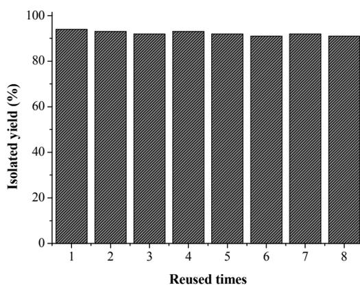
**Fig. 3** Recycle of the MCM-41-1,10-Phen-CuI catalyst.
