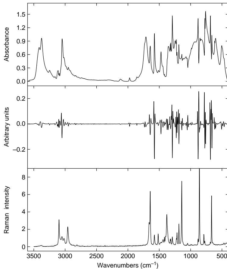
Fig. 5. Vibrational spectra: (a) FTIR spectra (suspension in Nujol and Fluorolube) of  $(\text{MIN})_2\text{H}\cdot\text{Cl}\cdot\text{H}_2\text{O}$ ; (b) second derivative FTIR spectrum and (c) Raman spectrum.
