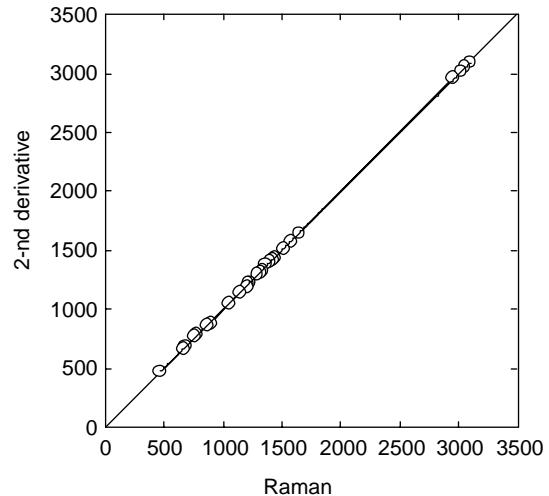
Fig. 6. Relation between  $d^2$  and Raman frequencies for (MIN)<sub>2</sub>H·Cl·H<sub>2</sub>O;  $y(d^2) = 3.0243 + 0.9980 v(\text{Raman})$ ,  $r = 0.9998$ .
