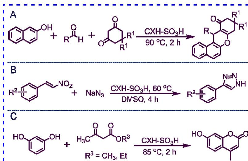
**Scheme 1** The CXH-SO<sub>3</sub>H was applied in the synthesis of benzoxanthenes (A), 4-aryl-NH-1,2,3-triazoles (B), and 7-hydroxy-4-methylcoumarin (C).
