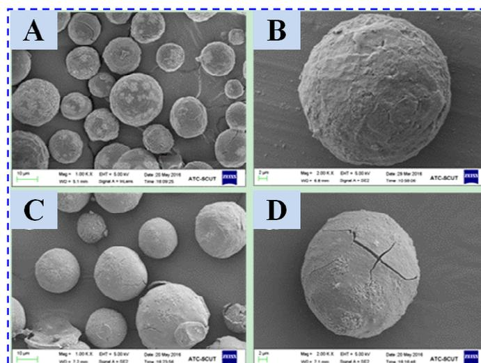
**Fig. 4.** SEM images of fresh CXH-SO<sub>3</sub>H (A and B) and the fifth reused of CXH-SO<sub>3</sub>H (C and D)
