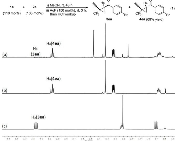
**Figure 1.** <sup>1</sup>H NMR studies of the stereochemistry (illustrating from 1.5–3.5 ppm). Spectrum (a) refers to the diastereoisomeric mixture resulting from eq 1; Spectrum (b) refers to major isomer from eq 1 after flash column chromatography; Spectrum (c) refers to the product **3ea** resulting from standard conditions.
