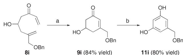
**Scheme 3** (a) **12** (7.5 mol%), toluene, 80 °C, 2 h; (b) ClCOCOCl, DMSO, Et<sub>3</sub>N, CH<sub>2</sub>Cl<sub>2</sub>, –78 °C, 1.5 h.
