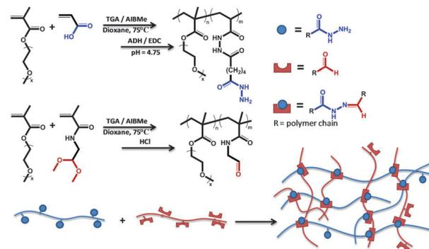
Scheme 1 Preparation of injectable PEG analogue hydrogels.
