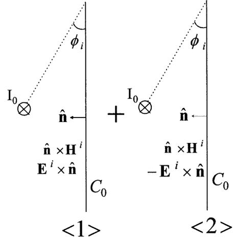
Fig. 2. The decomposition of PO currents.
