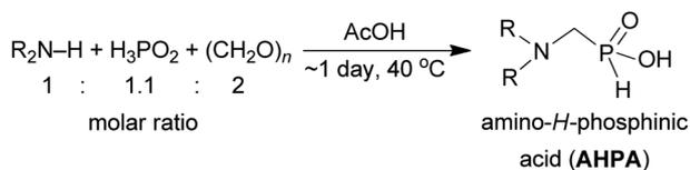
Scheme 1 Reaction of secondary amines, paraformaldehyde and  $\text{H}_3\text{PO}_2$ .
