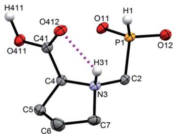
Fig. 4 Molecular structure of **13** found in the crystal structure of  $13 \cdot 0.25\text{H}_2\text{O}$ . Magenta dashed line shows intramolecular hydrogen bond. Carbon-bound hydrogen atoms are omitted for sake of clarity.
