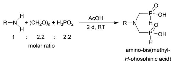
**Scheme 3** Reaction of primary amines, paraformaldehyde and H<sub>3</sub>PO<sub>2</sub>.
