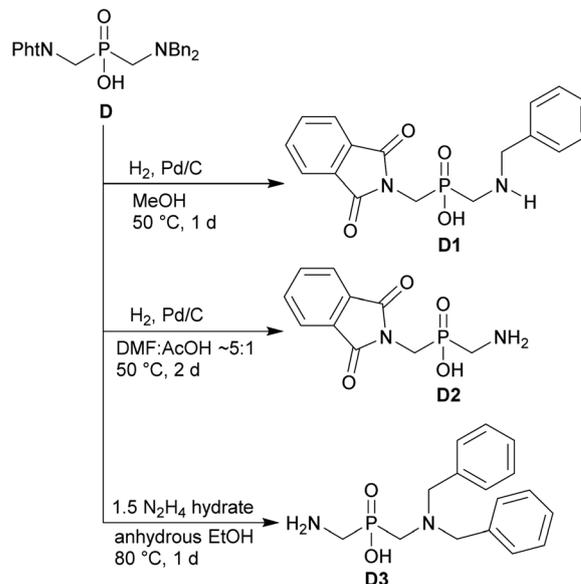
Scheme 9 Orthogonal protection of the amine groups in (NH<sub>2</sub>CH<sub>2</sub>)<sub>2</sub>PO<sub>2</sub>H.
