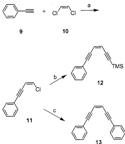
Scheme 1. Synthesis of **12** and **13**: a) Pd(PPh<sub>3</sub>)<sub>4</sub>, CuI, *n*BuNH<sub>2</sub>, C<sub>6</sub>H<sub>6</sub>, room temp., 24 h, 76%; b) TMS-acetylene (1.3 equiv.), Pd(PPh<sub>3</sub>)<sub>4</sub>, CuI, *n*BuNH<sub>2</sub>, C<sub>6</sub>H<sub>6</sub>, room temp., 48 h, 84%; c) **9** (1.0 equiv.), Pd(PPh<sub>3</sub>)<sub>4</sub>, CuI, *n*BuNH<sub>2</sub>, C<sub>6</sub>H<sub>6</sub>, room temp., 24 h, 87%
