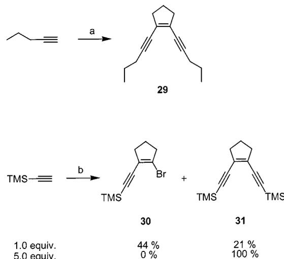
Scheme 9. Synthesis of **29**, **30** and **31**: a) **20** (0.25 equiv.), PdCl<sub>2</sub>(PPh<sub>3</sub>)<sub>2</sub>, CuI, *n*BuNH<sub>2</sub>, C<sub>6</sub>H<sub>6</sub>, room temp., 48 h, 87%; b) **20**, PdCl<sub>2</sub>(PPh<sub>3</sub>)<sub>2</sub>, CuI, *n*BuNH<sub>2</sub>, C<sub>6</sub>H<sub>6</sub>, room temp., 18 h
