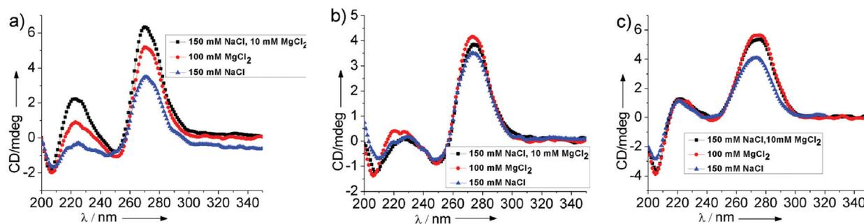
**Fig. 4** Effect of magnesium ions on folding of (*S*)-BuNA duplexes. (a) ON-1/ON-2. (b) ON-5/ON-6. (c) ON-8/ON-10. Experimental conditions: [oligonucleotide] = 5  $\mu$ M, 10 mM phosphate buffer containing 150 mM NaCl at pH 7.0; 10 mM tris buffer containing 100 mM MgCl<sub>2</sub> or 10 mM MgCl<sub>2</sub>, 150 mM NaCl at pH 7.
