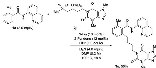
Scheme 2 Access to benzamide bearing a nitrogen-rich xanthine core.
