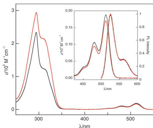
**Fig. 1** Absorbance spectra ( $\text{CHCl}_3$ ) of **1** (black) and **2** (red). Inset shows the absorbance and photoluminescence in the quinacridone region.
