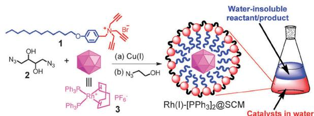
**Fig. 1** Preparation of the SCM-encapsulated rhodium catalyst and schematic representation of the biphasic catalytic hydrogenation of water-insoluble alkenes in water.
