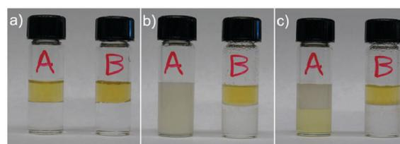
**Fig. 2** Comparison of rhodium complex **3** protected by CTAB (A) and SCM (B) in the presence of  $\text{CHCl}_3$  (a) before, (b) after 2 min of hand-shaking and 1 min of standing, and (c) after standing overnight at room temperature.
