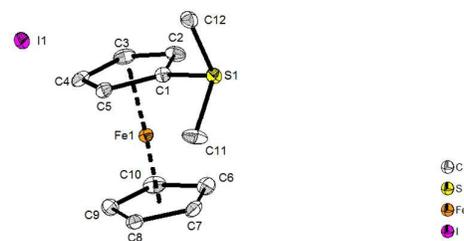
**Figure 4.** Molecular structure of **4**, hydrogen atoms omitted for clarity. Relevant bond distances per Å and angles per  $^\circ$ : S1-C1: 1.754(2), S1-C11: 1.793(3), S1-C12: 1.796(2), C1-C2: 1.433(3), C2-C3: 1.413(3), C3-C4: 1.427(3), C4-C5: 1.413(3), C1-C5: 1.435(3), S1-C1-C2: 122.96(16), S1-C1-C5: 128.16(15), Fe1-Cp(SMe<sub>2</sub>): 1.6642(3), Fe1-Cp': 1.6558(3).
