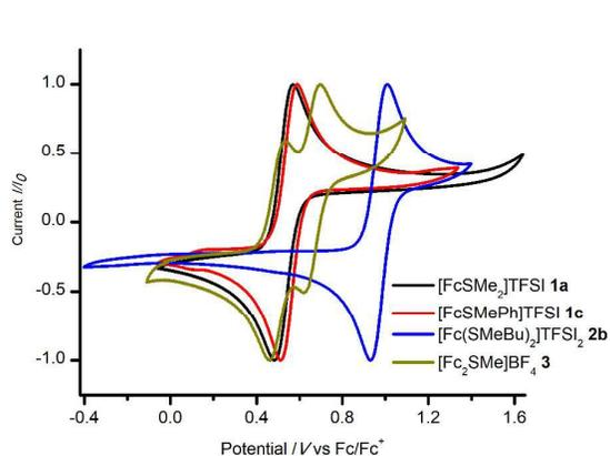
**Figure 3.** Cyclic voltammograms of selected new ferrocenylsulfonium compounds plotted against  $Fc/Fc^+$ . The measurements were performed in [EMIM]TFSI with an Ag/AgTFSI reference electrode with a scan rate of  $10 \text{ mV s}^{-1}$  for compounds **1a**, **1c**, **2b**. In case of compound **3** a scan rate of  $50 \text{ mV s}^{-1}$  was chosen because of better peak separation.
