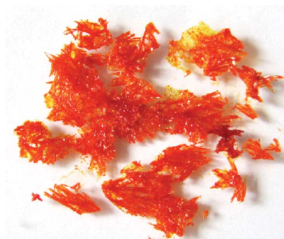
Fig. 1 Crystals of 1,4-bis(3-methylimidazolium-1-yl)butane ditribromide [bMImB]·(Br 3 ) 2 .
