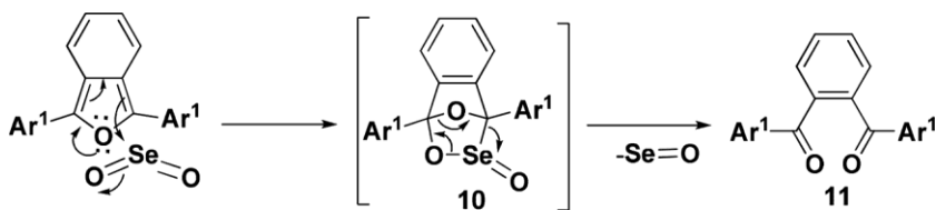
Scheme 1. Mechanism for oxidative cleavage of 1,3-disubstituted benzo[ c ]furans using \text{SeO}_2
