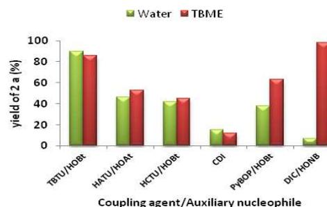
**Fig. 3** A comparison of yield of 2a in H<sub>2</sub>O and TBME in various coupling reagents
