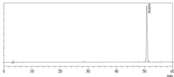
**Fig. 6** HPLC chromatogram of pentagastrin (5a). Method: C-18, 300 Å, 5 μm, 250×4.6 mm column, run for 60 min with a flow of 1 mL/min, using a gradient of 95–5%, where buffer A was 0.1% TFA in H<sub>2</sub>O and buffer B was 0.1% TFA in CH<sub>3</sub>CN and detection at 220 nm
