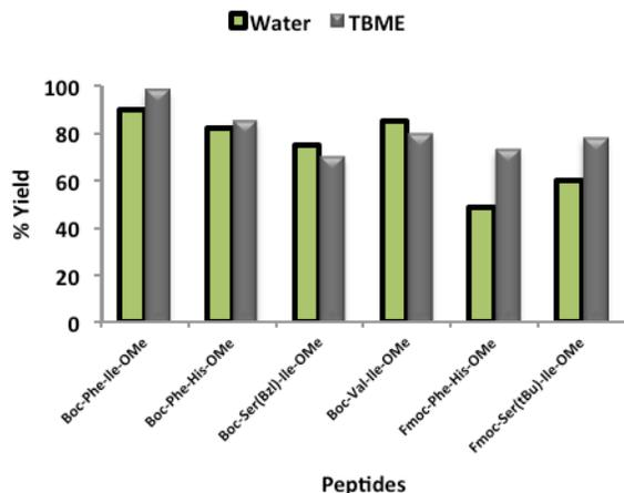
**Fig. 4** Reaction conditions: (a) H<sub>2</sub>O (2.5 mL), 1a (1.2 equiv), 1b (1.0 equiv), TBTU (1.2 equiv), HOBT (1.2 equiv), DIEA (2 equiv), 60 °C, 30 min, MW; (b) TBME (2.5 mL), 1a (1.2 equiv), 1b (1.0 equiv), DIC (1.2 equiv), HONB (1.2 equiv), DIEA (2 equiv), 60 °C, 30 min, MW.
