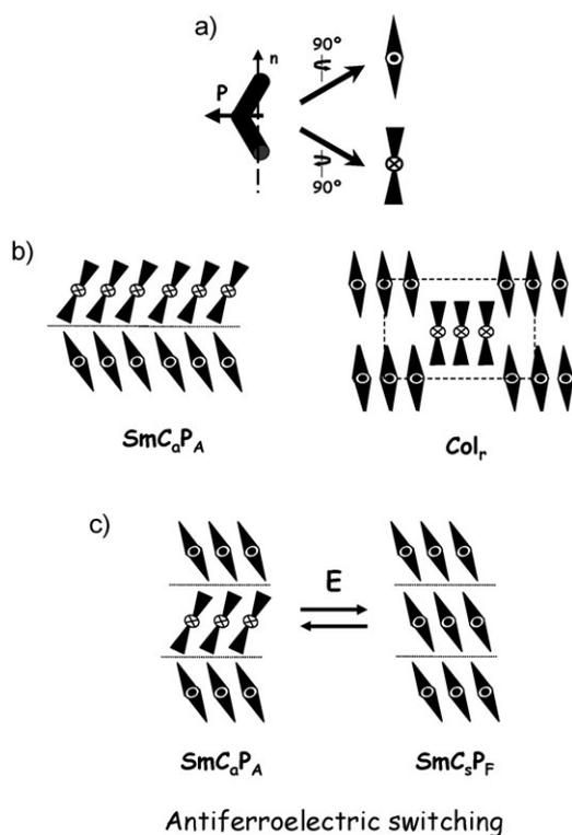
**Fig. 2** Schematic representations used for bent-shaped molecules (a). Models proposed for some of the arrangements, in the SmCP and Col<sub>r</sub> packings (b). Schematic representations of the antiferroelectric switching of a SmC<sub>d</sub>P<sub>A</sub> and SmC<sub>s</sub>P<sub>F</sub> mesophase induced by applying an electric field (c).
