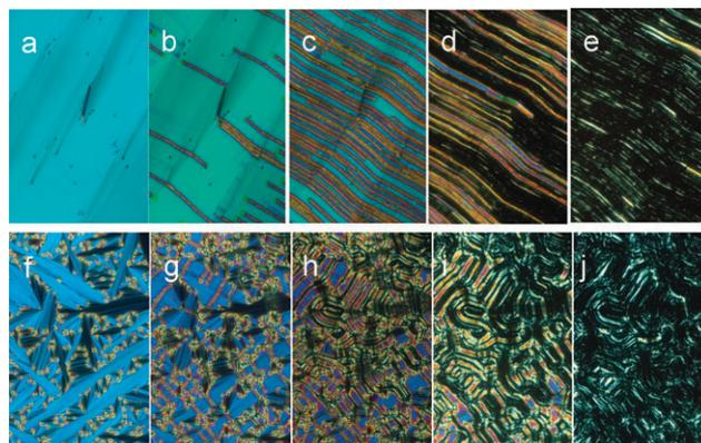
**Fig. 5** Microphotographs in 5 µm commercial Linkam cell of compounds: (top) **N(2,3)** at 207 °C applying no electric field (a) and applying (b) 120 V<sub>pp</sub>, (c) 130 V<sub>pp</sub>, (d) 140 V<sub>pp</sub> and (e) 150 V<sub>pp</sub> of AC voltage at 1 Hz; (bottom) **N(1,2)** at 164 °C applying no electric field (i) and applying (j) 200 V<sub>pp</sub>, (k) 220 V<sub>pp</sub>, (l) 230 V<sub>pp</sub> and (e) 240 V<sub>pp</sub>.
