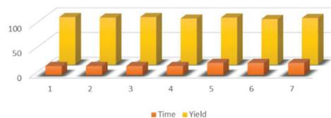
**Fig. 8** The reusability of the catalyst for a series of seven consecutive runs of the reaction of *N*-phenylmaleimide (0.3 mmol), *N,N*-dimethylaniline (0.45 mmol) and CdS as a nano-photocatalyst (10 mol%) under LED 12 W lamp irradiation and solvent-free conditions at room temperature.
