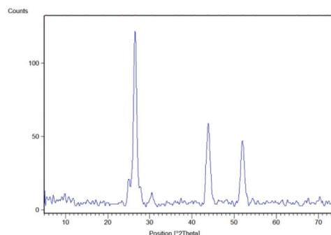
Fig. 2 The XRD patterns of freshly synthesized CdS NPs.
