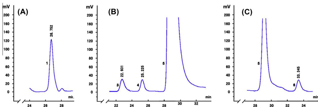
**Fig. 2.** Semi-prep HPLC chromatogram of compound 1 (A), compound 3, compound 4 and compound 5 (B), and compound 6 (C). Experimental conditions: column, Phenomenex  $C_{18}$  column (250 × 10.0 mm, 8  $\mu$ m); mobile phase, methanol–water (12:88, v/v) (A), methanol–water (11:89, v/v) (B) and methanol–water (10:90, v/v) (C), respectively; flow rate, 4.0 ml/min; detection wavelength, 275 nm; column temperature, 25 °C.
