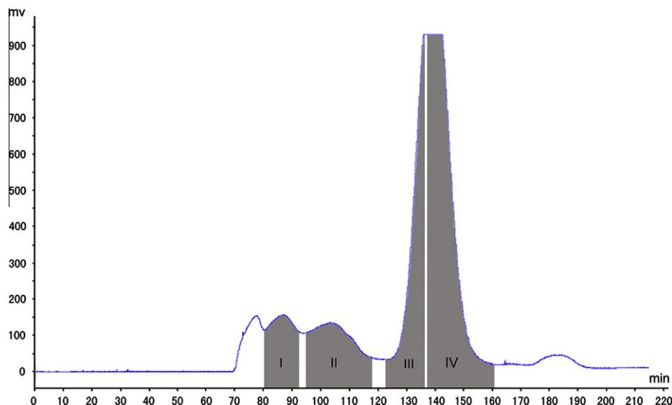
**Fig. 1.** HSCCC chromatogram of the crude extract from *R. crenulata*. Experimental conditions: two-phase solvent system, ethyl acetate–*n*-butanol–water (0.5:4.5:5, v/v/v); stationary phase, upper phase; mobile phase, lower phase; elution mode, head to tail; flow rate, 2.0 ml/min; revolution speed, 850 rpm; separation temperature, 30 °C; detection wavelength, 280 nm; sample loading, 150 mg/20 ml; retention of stationary phase: 68.9%.
