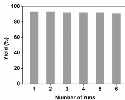
**Fig. 5** Reusability of the magnetic catalyst Nanocat-Fe-Ce.
