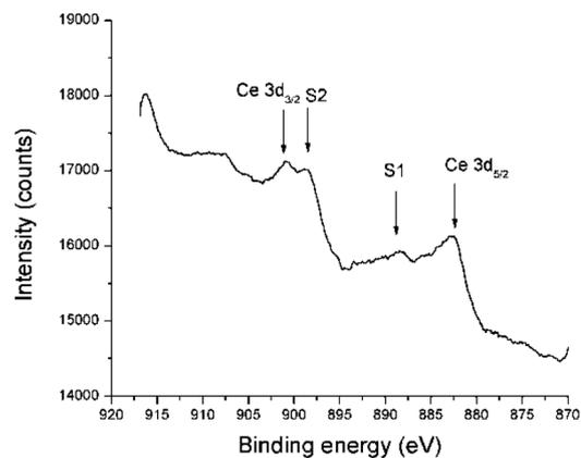
**Fig. 4** The Ce 3d line taken from the Nanocat-Fe-Ce powder. The expected positions of the main Ce  $3d_{5/2}$  line, its satellite peaks (S1 and S2) and the main Ce  $3d_{3/2}$  line in the case of  $\text{CeO}_2$  compound<sup>30,31</sup> are marked by arrows.
