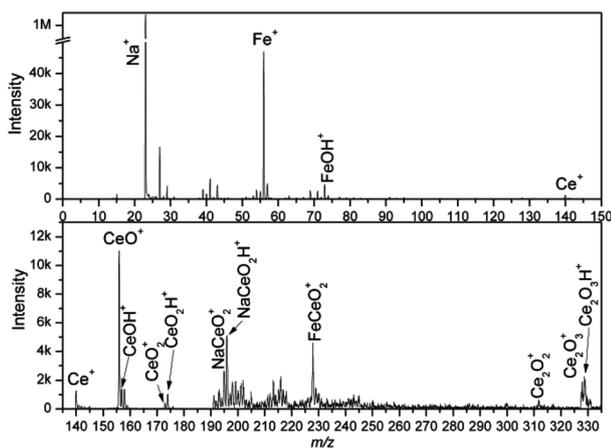
**Fig. 3** TOF-SIMS spectra of Nanocat-Fe-Ce MNPs (positive mode): top spectrum  $m/z$  range 0–150, and bottom spectrum  $m/z$  range 135–355.
