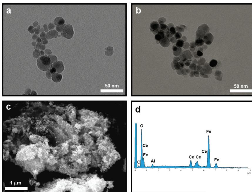
**Fig. 2** Characterization of the MNPs: (a) TEM image of  $\text{Fe}_3\text{O}_4$ ; (b) TEM image of Nanocat-Fe-Ce; (c) SEM image of Nanocat-Fe-Ce; (d) EDS profile of Nanocat-Fe-Ce.
