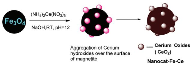
Scheme 1 Synthesis of Nanocat-Fe-Ce by wet impregnation.
