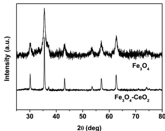
Fig. 1 XRD patterns of  $\text{Fe}_3\text{O}_4$  and Nanocat-Fe-Ce MNPs.
