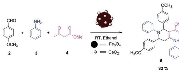
**Scheme 2** Synthesis of methyl 2,6-bis(4-methoxyphenyl)-1-phenyl-4-(phenylamino)-1,2,5,6-tetrahydropyridine-3-carboxylate (**5**).
