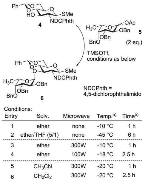
**Scheme 1.** Synthesis of disaccharide **6**. Microwave irradiation in low temperatures gave fruitful results. (a) Observed temperatures by the CoolMate equipped sensor with the use of microwave irradiation, within  $\pm 5$  °C. (b) The reactions were monitored by TLC and stopped when acceptor (**6**) was consumed.
