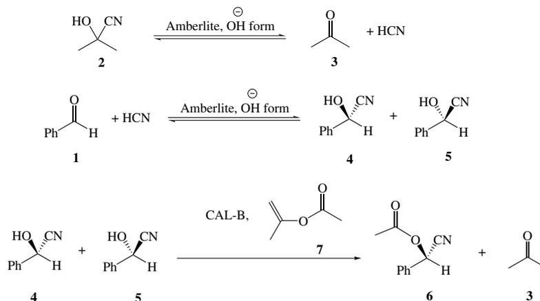
**Scheme 1.** Enantioselective synthesis of cyanohydrins by a dynamic kinetic resolution. All reactions proceed simultaneously in one pot.
