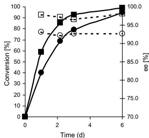
**Figure 2.** Dynamic kinetic resolution according to Scheme 1 utilising 1350 U/mmol CAL-Bcel (■ % **6** formed; □ ee of **6**) or CAL-Bpma (● % **6** formed; ○ ee of **6**).
