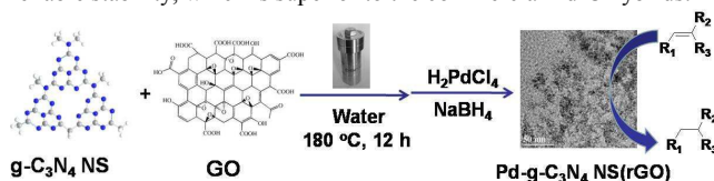
Scheme 1 Schematic illustration of the preparation process of the Pd-g-C 3 N 4 NS/rGO catalyst.
