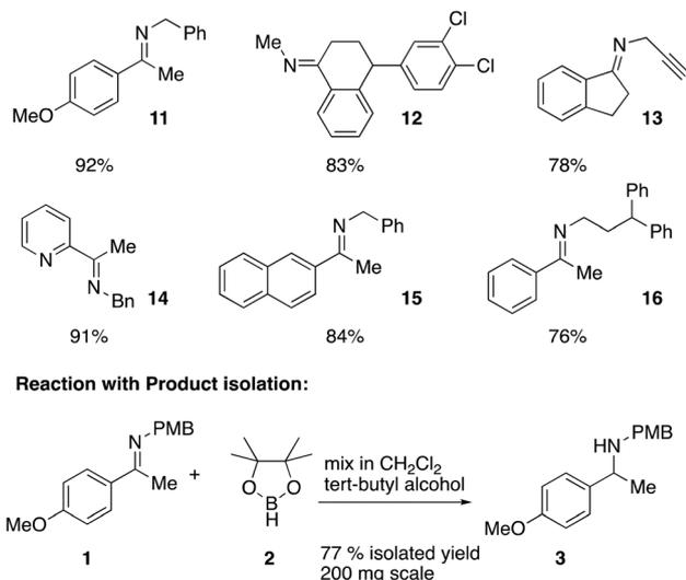
**Scheme 4** Imines reduced with *tert*-butyl alcohol/pinacolborane (NMR yields from integration with internal standard).
