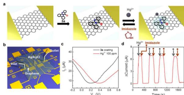
**Fig. 1** (a) Schematic illustration. (b) Graphene-FET sensor. (c) Transfer ( $I_D$ - $V_G$ ) characteristics ( $V_D = 0.1$  V). (d) Highly reversible  $Hg^{2+}$  sensing.
