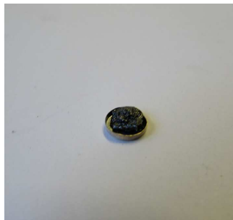
Epoxy polymer from GS lignin model mixture after TGA
