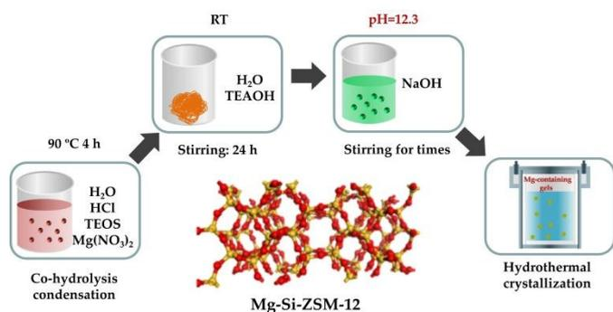
Scheme 1 Schematic illustration of the synthesis procedure and structural skeleton of Mg-Si-ZSM-12.
