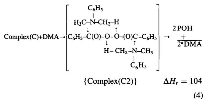
The formation of Complex(C2) assumed explains also the deceleration of the overall reaction experienced in apolar solvent (benzene) since the formation of radicals occurs only after two ionic steps.
