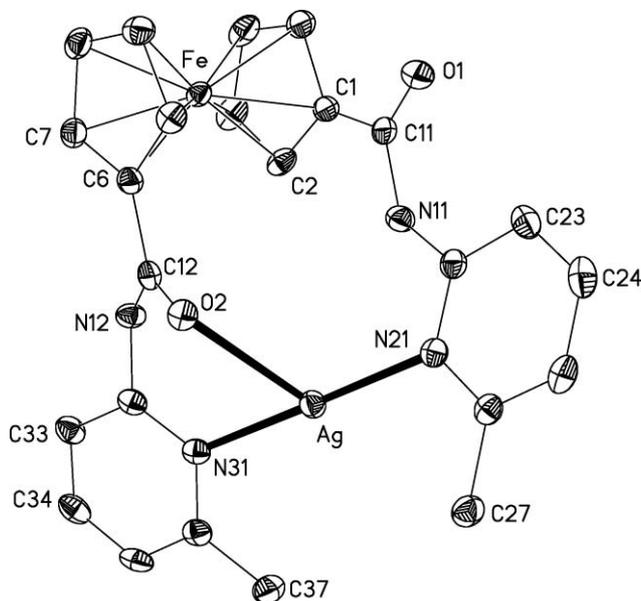
Fig. 3 Perspective view of the X-ray structure of the cation of complex **5** showing the atom labelling scheme. Hydrogen atoms have been omitted for clarity. Ellipsoids represent 50% probability levels.
