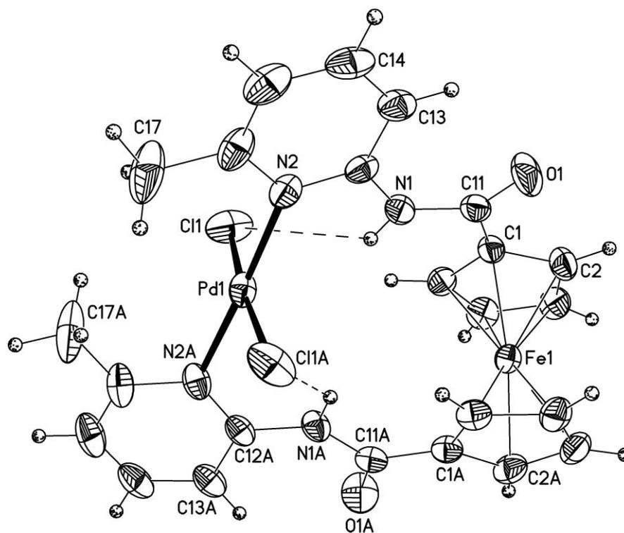
Fig. 5 Molecular structure of compound **11** showing the atom numbering scheme. Displacement parameter ellipsoids represent 50% probability surfaces.
