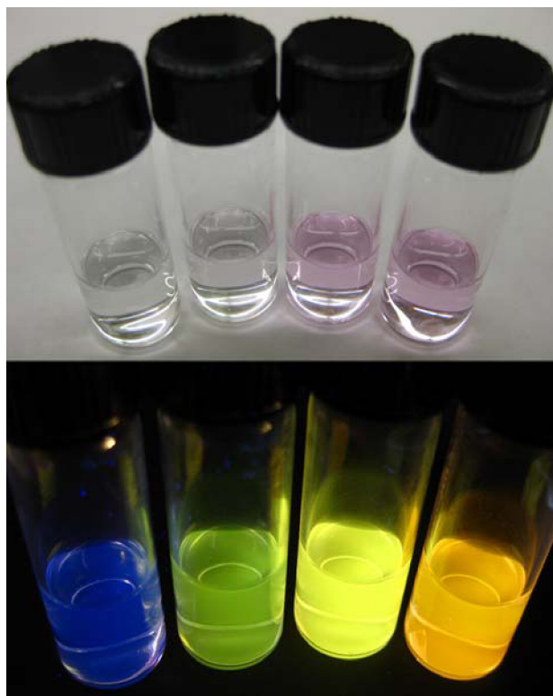
Figure 8. Photographs show the color of a \text{CH}_3\text{CN} solution of 4 (top, 10 \mu\text{M} ) and the fluorescence emission (bottom) upon illuminating the same sample using a hand-held UV lamp ( \lambda_{\text{ex}} = 365 \text{ nm} ) in the presence of various equiv of \text{Zn}(\text{ClO}_4)_2 , from left to right: 0, 1.5, 3, 10 equiv.
