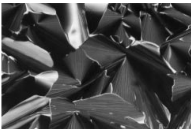
Figure 4. Optical texture of the hexagonal columnar mesophase of compound 4 as obtained by cooling from the isotropic melt (crossed polarizers) at 30 °C.
