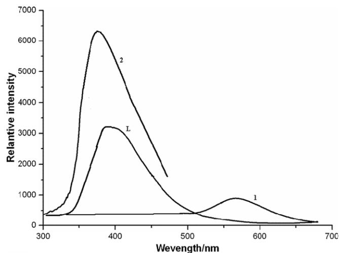
Fig. 10. Emission spectra of **1**, **2**, and free ligand  $H_2poda$  (L) in solid-state at room temperature.
