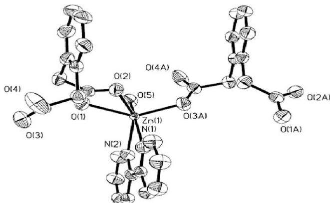
**Fig. 3.** The coordination environment of Zn in compound **2**.
