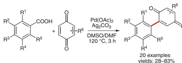
**Scheme 1** Synthesis of aryl-substituted 1,4-benzoquinones using arene carboxylates and 1,4-benzoquinone
