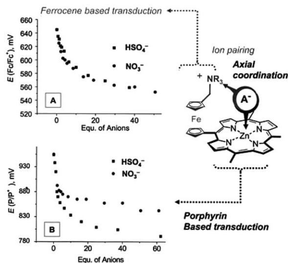
**Fig. 4** Evolution of (A) the ferrocene-based and (B) the porphyrin-based DPV oxidation peak potentials for  $[\mathbf{1}]^+ \cdot \text{BF}_4^-$  ( $5 \times 10^{-4}$  M) as a function of added molar equivalents of  $\text{TBANO}_3$  and  $\text{TBAHSO}_4$ .
