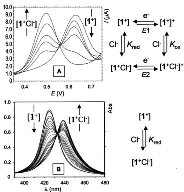
**Fig. 6** Evolution of (A) the DPV peak (scan rate 10 mV s<sup>-1</sup>, same conditions as in Fig. 3) and (B) the Soret visible absorption band (4.8 × 10<sup>-6</sup> M, CH<sub>2</sub>Cl<sub>2</sub>, 0.1 M TBAP) of [I]<sup>+</sup>·BF<sub>4</sub><sup>-</sup> as a function of added chloride (0 to 1 and 0 to 500 equiv. for A and B, respectively). The equilibria involved in these evolutions are depicted to the right of the titration curves.
