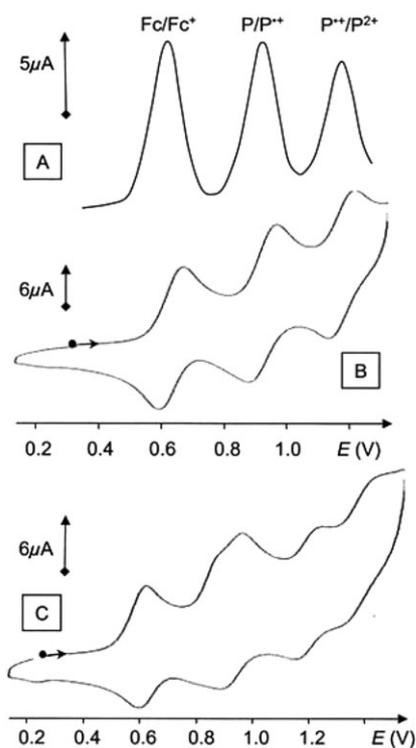
**Fig. 3** Differential pulsed (A) and cyclic (B) voltammograms of a  $5 \times 10^{-4}$  M  $\text{CH}_2\text{Cl}_2$  (TBAP, 0.1 M) solution of  $[\mathbf{1}]^+$ ,  $\text{BF}_4^-$ ; (C) cyclic voltammogram of a  $5 \times 10^{-4}$  M  $\text{CH}_2\text{Cl}_2$  (TBAP, 0.1 M) solution of  $\mathbf{2}$ ; 3 mm diameter carbon working electrode;  $\nu = 100 \text{ mV s}^{-1}$  (CV) and  $10 \text{ mV s}^{-1}$  (DPV);  $E(\text{V})$  vs.  $[\text{Fe}(\text{Cp}^*)_2]^{0+}$ .
