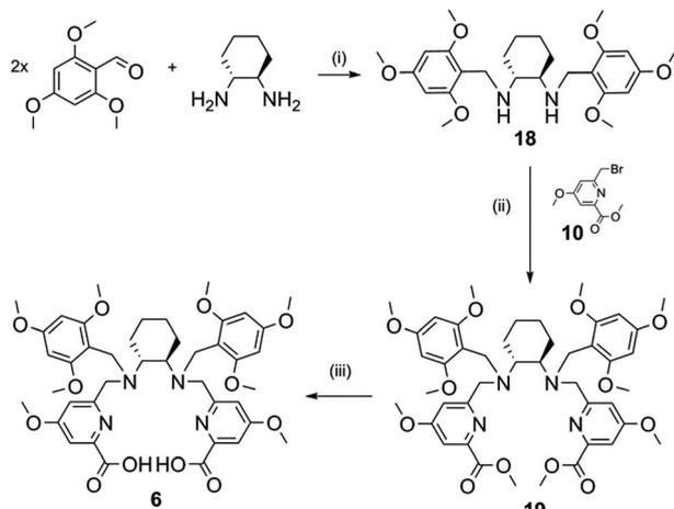
**Scheme 3** Synthesis of pro-ligand  $\text{H}_2\text{CHXdedpa}_{\text{OMe-Bn}_{\text{OMe}}}$  (**6**). Reagents and conditions: (i) (a) ethanol,  $0^\circ\text{C}$  to RT, 18 h; (b)  $\text{NaBH}_4$ ,  $0^\circ\text{C}$ , 1.5 h; (ii) methyl-6-(bromomethyl)-4-methoxypicolinate (2.1 equiv.),  $\text{Na}_2\text{CO}_3$ ,  $\text{CH}_3\text{CN}$ , reflux to RT, 2 d. (iii) LiOH (5 equiv.), THF/ $\text{H}_2\text{O}$  (3 : 1), RT, 30 min.
