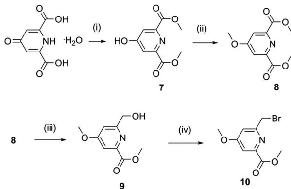
Scheme 4 Synthesis of precursors 7–10. Reagents and conditions: (i)  $\text{SOCl}_2$ ,  $\text{CH}_3\text{OH}$ ; (ii) methyl iodide,  $\text{K}_2\text{CO}_3$ ,  $\text{CH}_3\text{CN}$ , reflux; (iii)  $\text{NaBH}_4$ ,  $\text{CH}_3\text{OH}/\text{CH}_2\text{Cl}_2$  (2 : 1),  $0\text{ }^\circ\text{C}$ , 2 h; (iv) (1)  $\text{PBr}_3$ ,  $\text{CHCl}_3$ ,  $0\text{ }^\circ\text{C}$ –RT, 1.5 h, (2)  $0\text{ }^\circ\text{C}$ , aq  $\text{K}_2\text{CO}_3$ .
