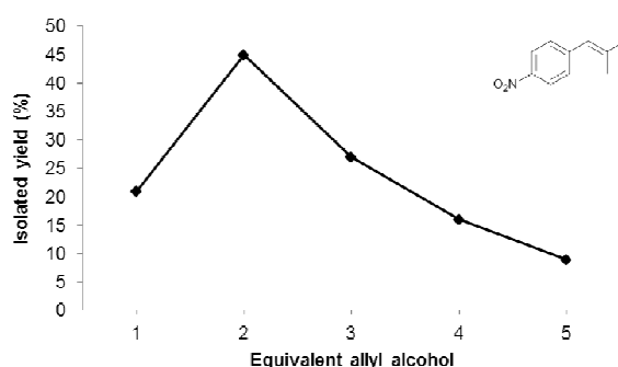
Figure 2 Effect of allyl alcohol excess on the reaction of 4-nitrobenzaldehyde with allyl alcohol. (Reaction conditions: 0.5 mmol aldehyde, 1 mL toluene, 5 mol% Pd (source: 5 % \text{Pd}/\text{Al}_2\text{O}_3 ), 0.5 mmol \text{K}_2\text{CO}_3 , 100^\circ\text{C} , 24 h.)
