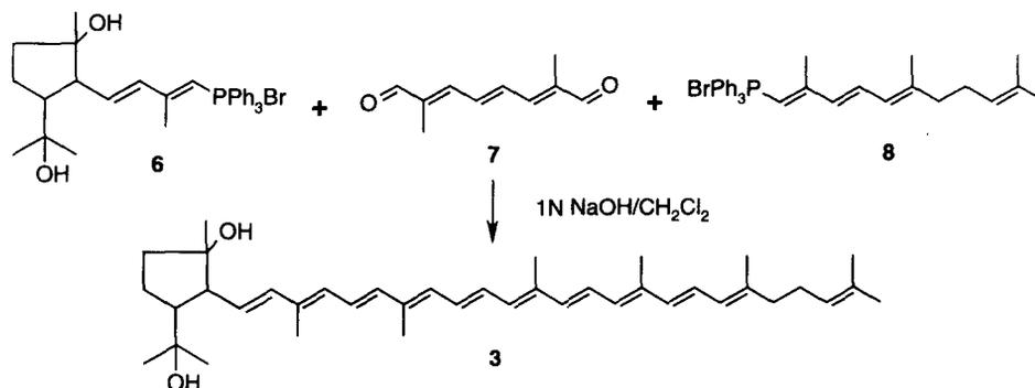
**Scheme 2:** Wittig olefination according to the strategy  $C_{15} + C_{10} + C_{15} = C_{40}$
