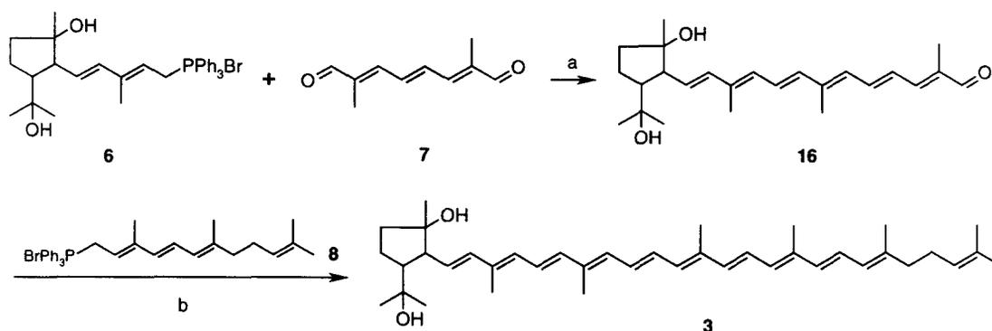
**Scheme 4:** Coupling of the central C<sub>10</sub>-building block **7** with the two C<sub>15</sub>-end groups **6** and **8**.
