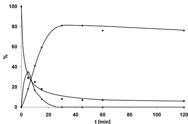
**Figure 1.** Yield *versus* time plot of the hydrosilylation of methyl linoleate **4** with chlorodimethylsilane **5**. ■: methyl linoleate **4**, ▲: conjugated methyl linoleate, ●: product **6**. 1 mol %  $\text{H}_2\text{PtCl}_6$ , further conditions as given in Table 2.
