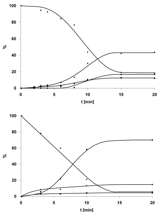
**Figure 2.** Yield *versus* time plot of the hydrosilylation of methyl undec-10-enoate **1** with triethoxysilane **2** in the solvent system cyclohexane/toluene/propylene carbonate. Conditions: 40 °C, equimolar amounts of **1** and **2**, 1 mol %  $\text{H}_2\text{PtCl}_6$  (above: first use, below: second use). ◆: methyl undec-10-enoate **1**, ■: isomerised methyl undecenoates, ▲: methyl undecanoate, ●: hydrosilylation product **3**.
