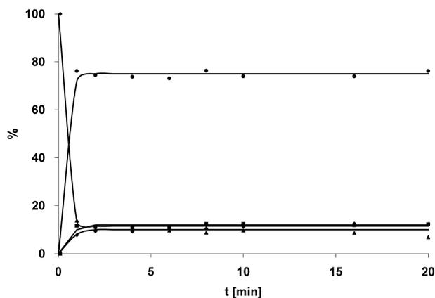
**Figure 3.** Yield *versus* time plot of the hydrosilylation of methyl undec-10-enoate **1** with triethoxysilane **2** in the solvent system cyclohexane/toluene/propylene carbonate. Conditions: 40 °C, equimolar amounts of **1** and **2**, 1 mol % Pt as Karstedt solution. ◆: methyl undec-10-enoate **1**, ■: isomerised methyl undecenoates, ▲: methyl undecanoate, ●: hydrosilylation product **3**.
