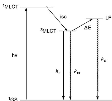
**Fig. 2** Energy state diagram based on the Crosby–Meyer model
