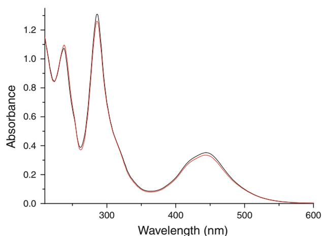
**Fig. 1** Absorption spectra of complexes [(bpy)<sub>8</sub>Ru<sub>4</sub>(L<sup>1</sup>)](PF<sub>6</sub>)<sub>8</sub> (black) and [(bpy)<sub>8</sub>Ru<sub>4</sub>(L<sup>2</sup>)](PF<sub>6</sub>)<sub>8</sub> (red) in CH<sub>3</sub>CN solution at room temperature. (Color figure online)
