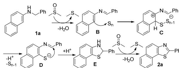
Scheme 4. Proposed reaction mechanism for the formation of **2a**
