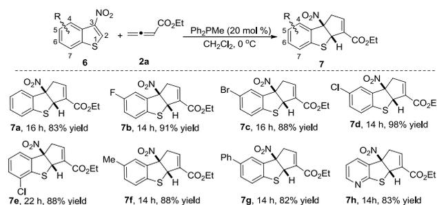
**Scheme 4** Substrates scope of 3-nitrobenzothiophenes. Reaction conditions: the reactions were carried out with **6** (0.15 mmol), **2a** (0.225 mmol) and  $\text{Ph}_2\text{PMe}$  (20 mol %) in 1.5 mL of  $\text{CH}_2\text{Cl}_2$  for indicated time.
