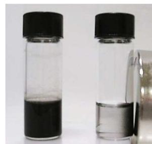
**Figure 3.** Left: nanohybrid catalyst suspension. Right: magnetic separation of CuFe<sub>2</sub>O<sub>4</sub>CNT (picture taken 15 seconds after the positioning of a permanent magnet).
