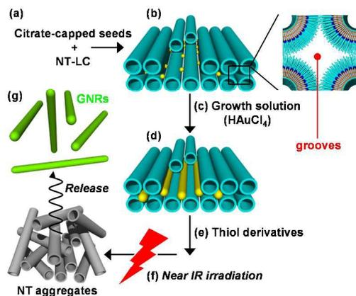
Fig. 2 Production of GNRs using NT-LC templates.
