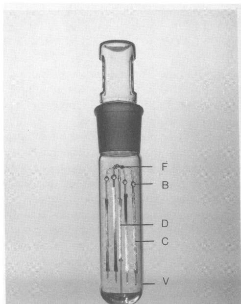
FIG. 1. Device for the determination of the affinity of various proteins for volatile organic compounds. V, glass vial (28 mm OD  $\times$  140 mm); F, five-pronged glass framework constructed from 1.0-mm glass rod and supported on the central prong; B, glass beads formed in the framework to keep the outer four prongs from touching the wall of the vial; D, dispensing glass-fiber wick treated with the volatile organic compound(s) under investigation; C, adsorbing wicks (collectors).
