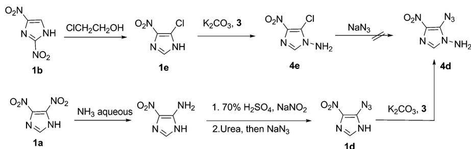
Scheme 2 Reaction optimization of 5-azido-4-nitroimidazole.
