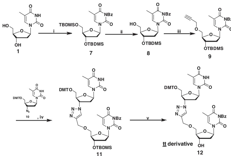
**Reagents:** i. (a) TBDMS-Cl/DMF 95% (b) Bz-Cl/pyridine 90% ii.  $I_2/MeOH$  70% iii. propargyl bromide, NaH/DMF 80%, iv. **10**, 0.2eq  $CuSO_4$ , 0.5eq Na-ascorbate *t*-BuOH: $H_2O$  80% v. 1M TBAF/THF, 87%
